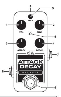
**Power Suppy Requirements:** Voltage: 9VDC Current: 100mA Polarity: Center-Negative This device comes equipped with an Electro-Harmonix 9.6DC-200 power supply. Use of the wrong adapter or a plug with the wrong polarity may damage the device and void the warranty. Do not exceed 10.5VDC on the power plug. Power supplies rated for less than 100mA may cause the device to act unreliably.
