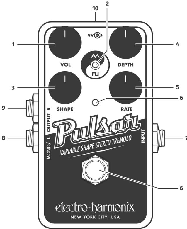
**1. VOL Knob** Adjusts the overall output level of the effect. As VOL is turned clockwise, the output gets louder. The VOL knob offers up to 12dB of volume boost depending on the settings of the other controls. When VOL is turned fully counter-clockwise the effect output is silenced.
