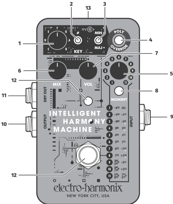
**1. KEY Knob** This seven-position rotary switch, in conjunction with the toggle switch to its right, sets the key the IHM is in while in Intelligent Mode. This knob has no effect while in Polyphonic Override Mode.
