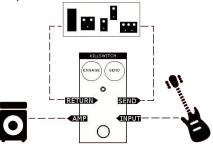
**INPUT JACK** – Connect to the output of your instrument or another effects pedal **SEND JACK** – Connect to the input of your effects loop
