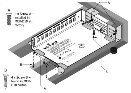
**A Screws: Please note**: the four A screws are installed into the sides of the MOP-D10 at the factory. Remove these screws, two at a time, then reinstall while attaching the brackets.
