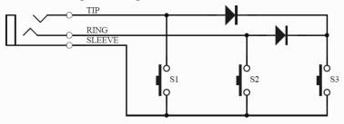
The switch connected to the TIP+RING of the external footswitch behaves like the BYPASS footswitch. Use this control to remotely switch the Superego+ on and off. This switch will also control triggers in LATCH mode.
