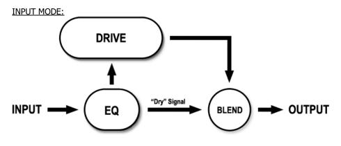
In INPUT mode the EQ comes first in the signal path, affecting both the clean signal and the signal fed into the distortion. Boosting frequencies in this mode can help drive the distortion signal to a more saturated tone.
