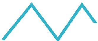
Triangle: An extra option just in the TREM type, the triangle wave is very similar to the sine, but with a slightly different feel as the parameter change is more linear.
