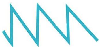
Falling Sawtooth: The opposite of the rising sawtooth, the modulated parameter smoothly falls from maximum to minimum, before sharply resetting at its maximum. Can be used for rhythmic effects.
