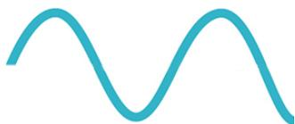
Sine: A sine wave LFO is the most common LFO shape and the default in every mod type in the MOD 11. The modulated parameter smoothly moves between its minimum and maximum in a fluid, seamless way.
