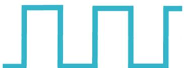
Square: The modulated parameter jumps directly between minimum and maximum, with no smooth transitions. Can be used to create choppy or robotic effects.
