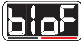
b1oF: 1-Shot mode is OFF for LOOP B
