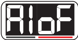
A1oF: 1-Shot mode is OFF for LOOP A
