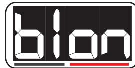
b1on: 1-Shot mode is ON for LOOP B
