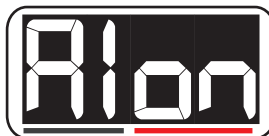
A1on: 1-Shot mode is ON for LOOP A
