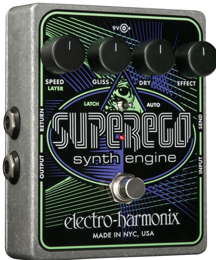
mode, you can hold whatever sound is played at the moment the effect switch is engaged, then improvise over it with a dry signal. If you press down on the footswitch again, an additional sound is layered on top of the previous sound. The number of layers, from one to infinity, can be selected with the speed/layer control. In Momentary mode, the speed/layer control adjusts the attack and decay of the “frozen” sound. In Auto mode, each new note, chord or sound played automatically
